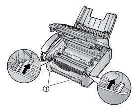
**3** Close the front cover (①) by pushing down on both sides, until locked.
